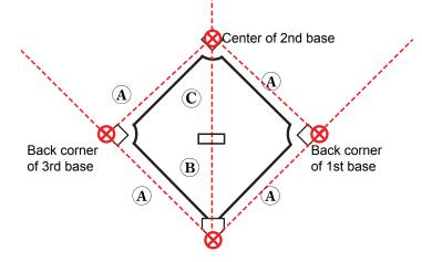
Dig 20" diameter hole no less than 10" deep for each base. Create a firm foundation using crushed stone or Baseball Clay at bottom of base. We suggest a minimum of 1 to 1-1/2" of material. Foundation should be tamped and leveled.
