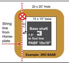
4. Backfill hole around PABF up to field level. Note: Top of Anchor should be 1" below field level. Rubber or Feathered Base Plugs are recommended if Base is not in place.
