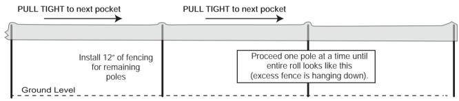
(D) Once you have successfully attached all of the required pockets, the material can be pulled down to the bottom end of each post. For best appearance, confirm that the fence is tightly stretched between each post and does not sag. Any excess fencing can be easily cut with sharp scissors.  $\mathcal{V}$
